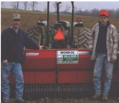
Drills and seeders have separate boxes so large and small seeds can be divided when planting. You can place them at different depths by making the proper adjustments on the drill.
