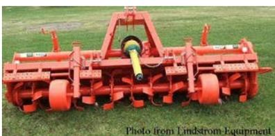
**Rotary hoe-** A rotary hoe (or rotovator) is similar to a large rototiller, but it operates from the power takeoff and three point hitch of a tractor. These units are generally used where finely tilled seedbeds are desired or where small plots are being installed. After tilling with a rotary hoe, use a cultipacker to firm the seedbed
