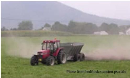
**Lime spreader-** Spreading lime is important if you need to increase soil pH. Applications rates of 2-3 tons per acre are not uncommon in Ohio so a large-capacity spreader may be necessary. Often, buggies may be rented from a local agricultural store or the Soil and Water Conservation District in your area if you have a tractor large enough to pull them. Agriculture commodity stores also have lime spreader trucks
