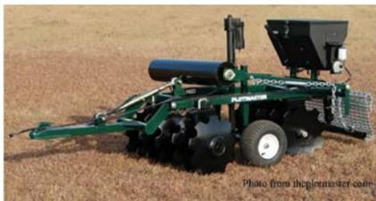
**Combination Tool-** Specialty type equipment is also available for those installing food plots with ATVs. This equipment is designed to carryout all steps necessary in preparing and planting seedbeds for food plots using various attachments designed for the tool.
